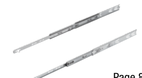
Telescopic slides, steel for surface mounting, over-extension, load capacity up to 60 kg K1579
