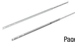
Telescopic slides, steel for slot mounting, partial extension, load capacity up to 10 kg K1566
