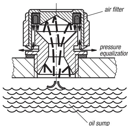
Gears partly immersed in an oil sump create an oil spray that may cause oil to leak from the vent cap. To avoid this the screw has been fitted with a splash guard. Only a small part of the oil spray can pass through the lower tapered bore. The oil that does reach the cap underside is redirected in such a way that it does not notably hinder the venting process.
